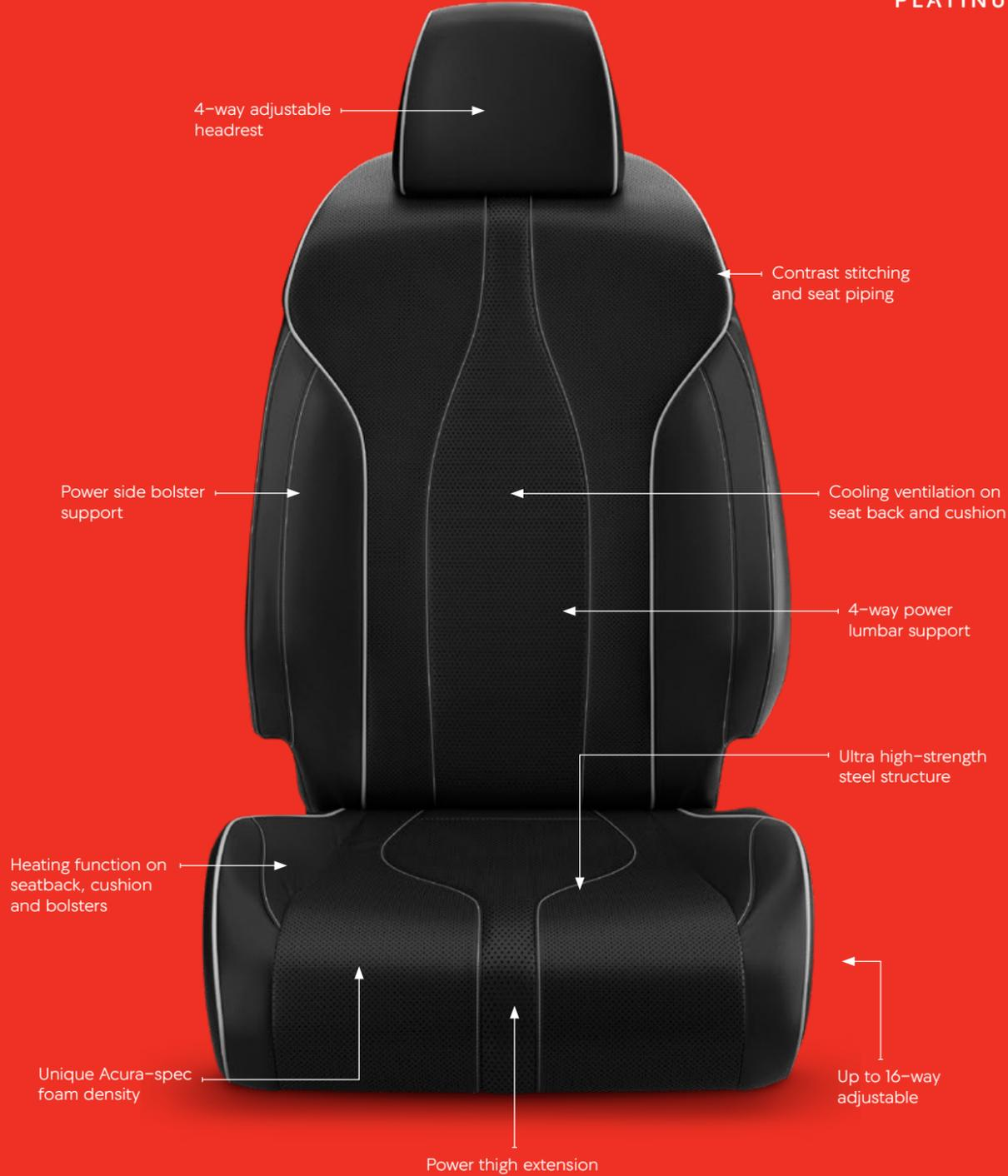
Even thrones don't hold this much power. Available 16-way power-adjustable front seats including 4-way power adjustable lumbar support, a 4-way adjustable headrest, a power thigh extension, a power side bolster support, heating and ventilated cooling were designed completely from scratch on a frame made from ultra-high-strength steel. Because the better the seat, the better the connection to the road.
